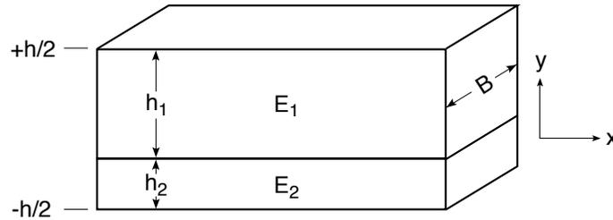
Fig. 2. The coordinate system used for composite beam analysis of one arm of an adhesive DCB specimen.
