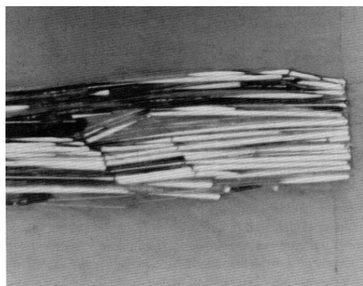
Figure 7: Typical cross sections of compression damage in composites having the fibers treated with release agent Frekote 700. The crosshead speed was 0.001 mm/sec. The magnification is 200X.
