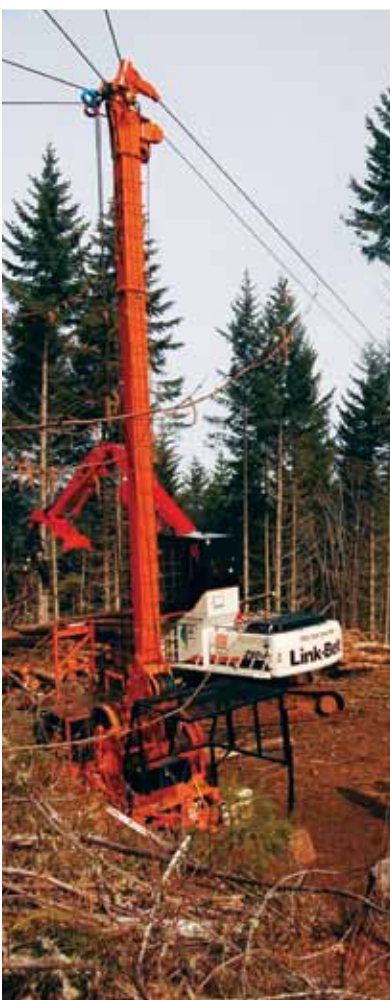
New yarder with the new log loader on site in McDonald-Dunn Forest. Photo credit: Talia Filipek (NR).
