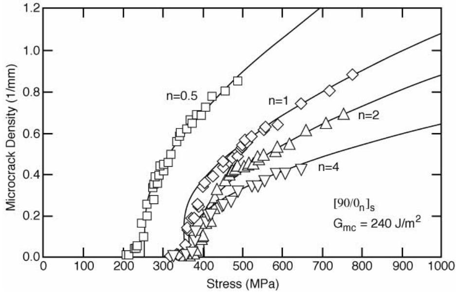
Fig. 14. Microcrack density as a function of applied load in a series of AS4/Hercules 3501-6 carbon/epoxy laminates. The symbols are experimental data points. The smooth lines are predictions using the variational mechanics energy release rate theory and  $G_{mc} = 240 \text{ J/m}^2$ .
