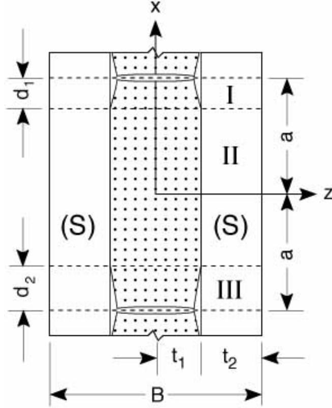
Fig. 19. Edge view of a  $[0_n/90_m]_s$  cross-ply laminate with microcracks and delaminations emanating from the tips of those microcracks. The dashed lines demarcate regions I, II, and III for the stress analysis.
