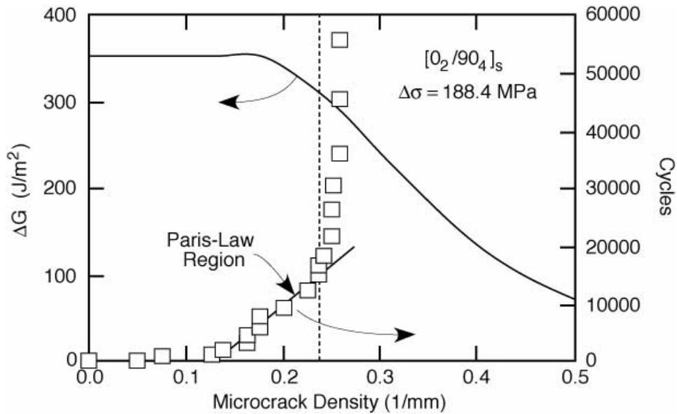
Fig. 16. Microcracking fatigue data for a  $[0_2/90_4]_s$  carbon/epoxy laminate. The solid line shows  $\Delta G$  as a function of microcrack density. The symbols show the microcrack density as a function of cycle number. The straight line through the microcrack density data shows the Paris-law region of constant microcrack density growth rate.
