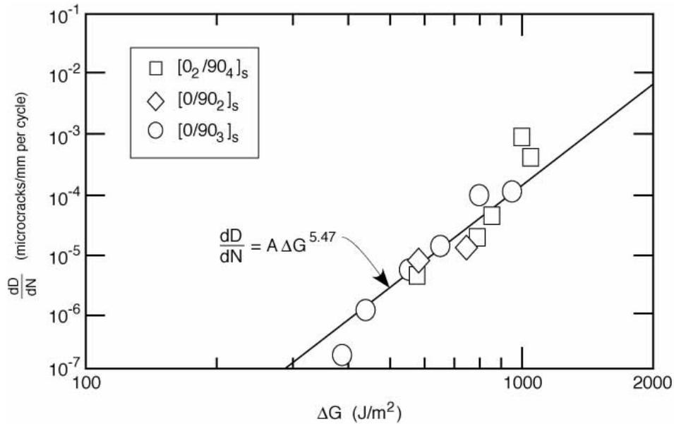
Fig. 17. The microcrack density growth rate (in microcracks per mm per cycle) as a function of applied  $\Delta G$  for Avimid<sup>®</sup> K Polymer/IM6 laminates. As indicated on the figure, the results are from three different cross-ply layups.
