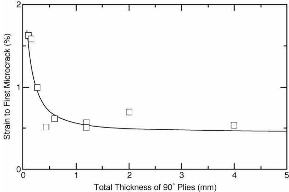
Fig. 2. The strain to initiate microcracking in E glass/Shell Epikote epoxy [0/90/0] laminates as a function of the total thickness of the 90° plies. The 0° plies each have a constant thickness of 0.5 mm. The data in from Ref. [13].
