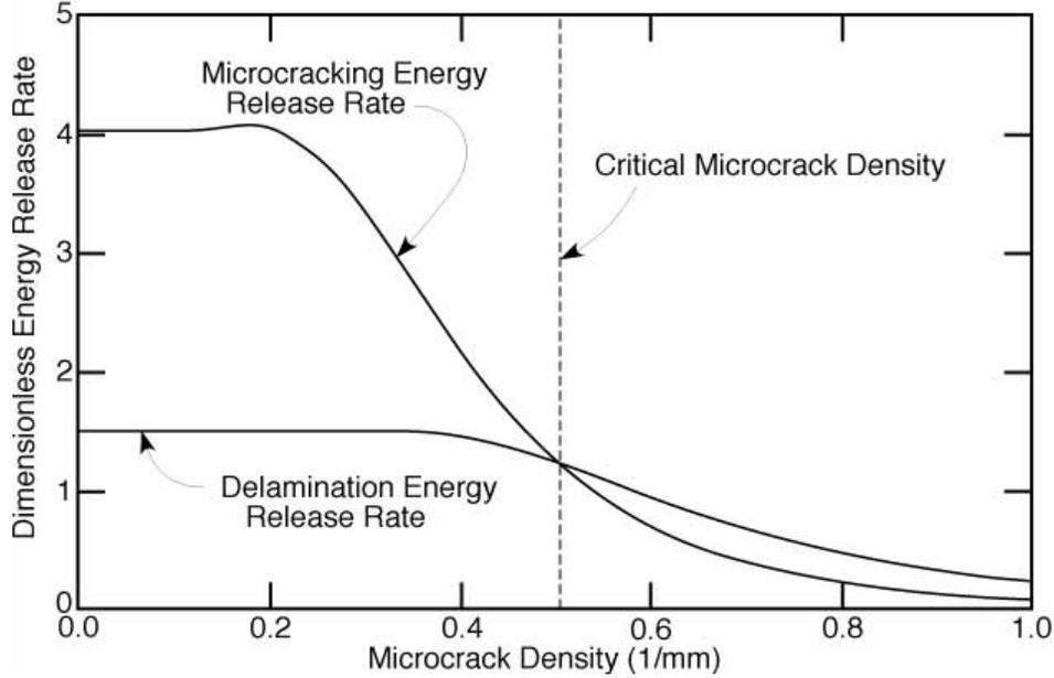
Fig. 20. Dimensionless energy release rates for initiation of delamination and for continued microcracking as functions of microcrack density for a  $[0_2/90_4]_s$  carbon/epoxy laminate. The critical microcrack density for delamination is defined by the microcrack density where the two curves cross.
