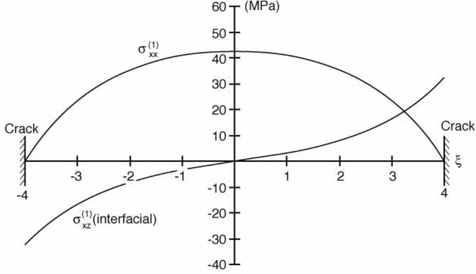
Fig. 8. Stresses between two microcracks in a  $[0/90_2]_s$  carbon/epoxy laminate from a one-dimensional analysis. The applied stress is 100 MPa, thermal load is  $T = -125^\circ\text{C}$ , and the microcrack spacing is  $\rho = 4$ . The normal stress ( $\sigma_{xx}^{(1)}$ ) is the average tensile stress in the  $90^\circ$  ply group. The plotted shear stress ( $\sigma_{xz}^{(1)}$ ) is the shear stress at the  $90/0$  interface.
