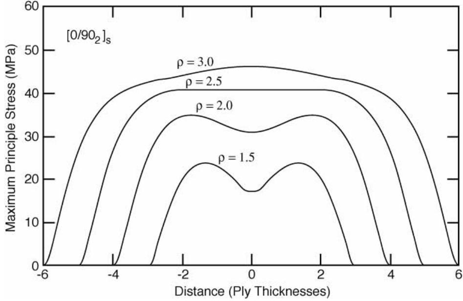
Fig. 21. The maximum principle stresses along the 90/0 interface in a  $[0/90_2]_s$  carbon/epoxy laminate for four values of the microcrack density.
