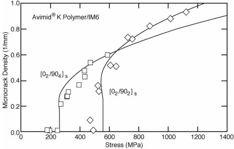
Fig. 3. The microcrack density as a function of applied load in IM6/duPont Avimid<sup>®</sup> K Polymer cross-ply laminates. The symbols are experimental data points and the smooth lines are predictions using an energy release rate approach and a variational mechanics stress analysis. Data and predictions are from Ref. [29].
