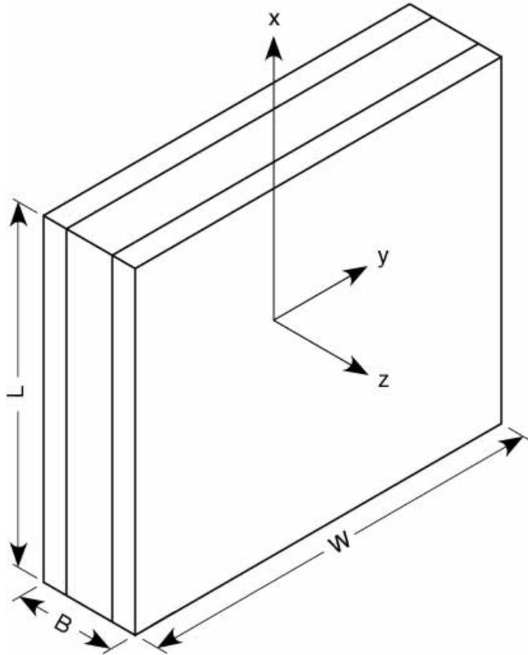
Fig. 5. The coordinate system for the stress analysis of  $[(S)/90_n]_s$  and  $[90_n/(S)]_s$  laminates.  $L$ ,  $W$ , and  $B$  are the length, width, and thickness of the laminate plate.
