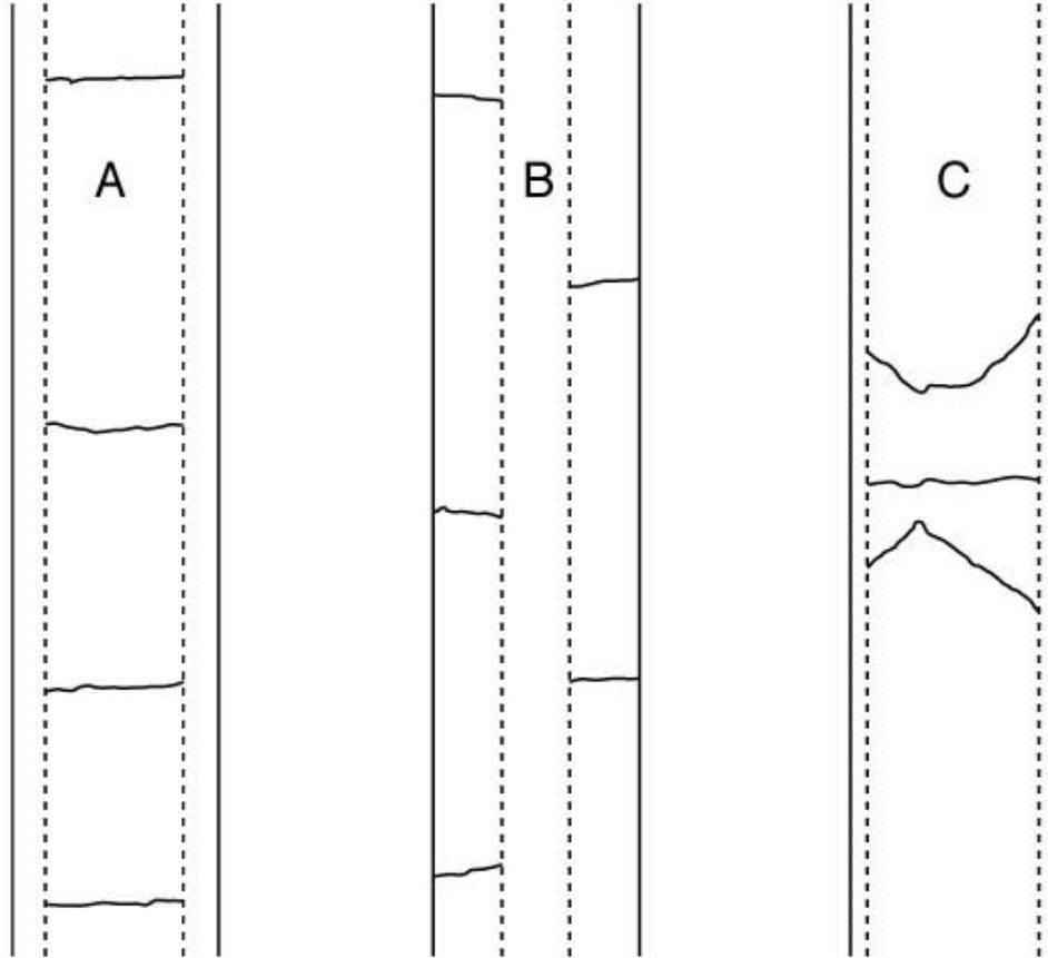
Fig. 4. Sketches of actual edge views of typically damaged cross-ply laminates. A. Roughly periodic array of microcracks in a  $[0/90_4]_s$  laminate. B. Antisymmetric or staggered microcracks in a  $[90_4/0_2]_s$  laminate. C. Two curved or oblique microcracks near one straight microcrack in a  $[0/90_8]_s$  laminate.
