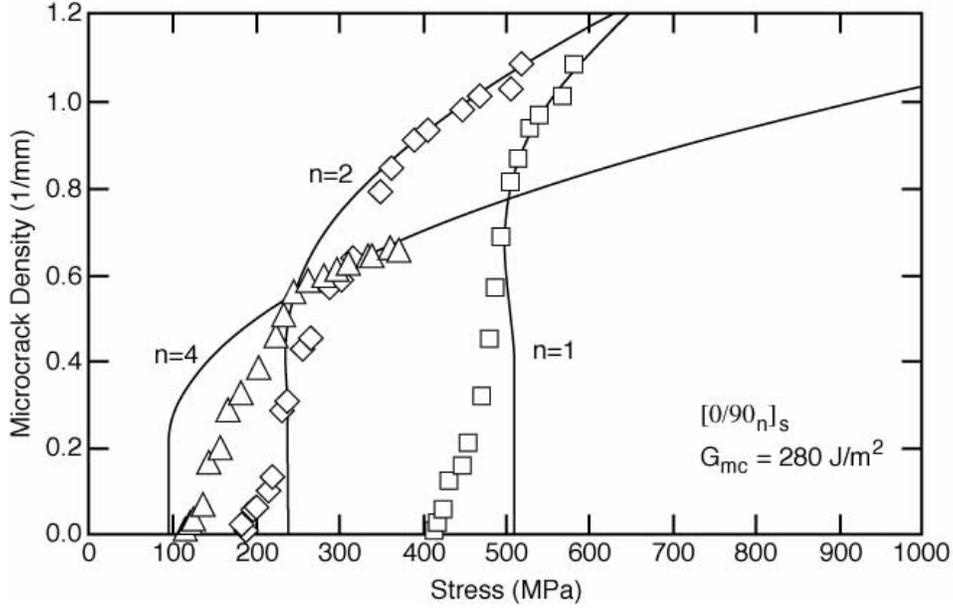
Fig. 12. Microcrack density as a function of applied load in a series of AS4/Hercules 3501-6 carbon/epoxy laminates. The symbols are experimental data points. The smooth lines are predictions using the variational mechanics energy release rate theory and  $G_{mc} = 280 \text{ J/m}^2$ .
