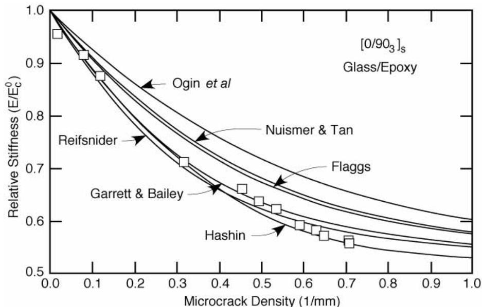
Fig. 11. Relative modulus as a function of microcrack density for a  $[0/90_3]_s$  glass/epoxy (Scotch Ply 1003) laminate. The data points are experimental results from Ref. [22]. The smooth lines are theoretical predictions by various stress analysis procedures.
