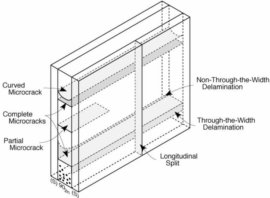
Fig. 1. A  $[0_n/90_m]_s$  laminates with several types of damage modes. The illustrated damage modes are complete microcracking, partial microcracking, microcrack induced delamination (both through-the-width delamination and non-through-the-width delamination that initiates at a free edge), curved microcracks, and longitudinal splitting
