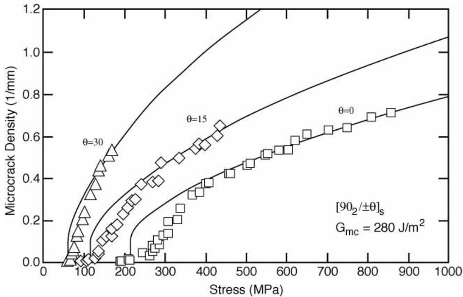
Fig. 15. Microcrack density as a function of applied load in a series of AS4/Hercules 3501-6 carbon/epoxy laminates. The symbols are experimental data points. The smooth lines are predictions using the variational mechanics energy release rate theory and  $G_{mc} = 280 \text{ J/m}^2$ .
