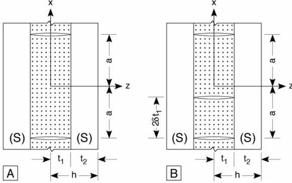
Fig. 6. Edge view of a  $[(S)/90_n]_s$  laminate with microcracks. A: Two microcracks in the  $90^\circ$  plies. B: The formation of a new microcrack at a distance  $2\delta t_1$  above the bottom microcrack.
