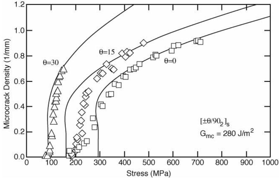
Fig. 13. Microcrack density as a function of applied load in a series of AS4/Hercules 3501-6 carbon/epoxy laminates. The symbols are experimental data points. The smooth lines are predictions using the variational mechanics energy release rate theory and  $G_{mc} = 280 \text{ J/m}^2$ .
