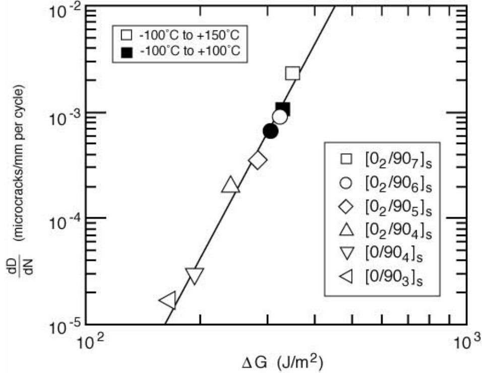
Fig. 18. The microcrack density growth rate (in microcracks/mm per cycle) as a function of applied  $\Delta G$  for AS4/Hercules 3501-6 during thermal cycling. As indicated on the figure, the results are from six different cross-ply layups and from two different thermal cycling temperature ranges.
