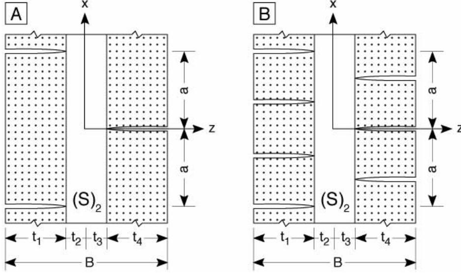
Fig. 7. A unit cell of damage in a  $[90_n/(S)]_s$  laminate having “staggered” or antisymmetric microcracks. A: A single unit cell of damage. B: Three unit cells of damage after formation of new microcracks at locations of local maxima in tensile stress.
