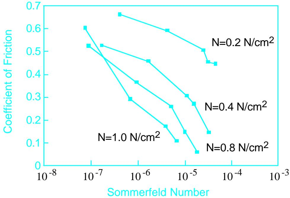
Figure 4: Coefficient of friction as a function of Sommerfeld number for a Bausch & Lomb SeeSequence® 2 Lens sliding on a PMMA disk while lubricated by a saline solution.
