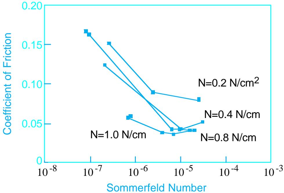
Figure 5: Coefficient of friction as a function of Sommerfeld number for a Johnson & Johnson NueVue® Lens sliding on a PMMA disk while lubricated by a saline solution.
