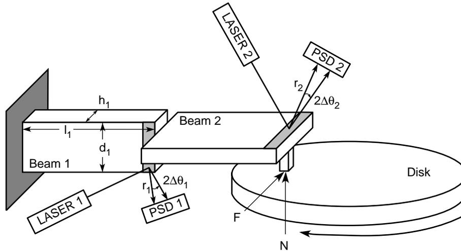
Figure 1: Schematic drawing of the main features of the pad-on-disk friction apparatus. The pad is attached to crossed cantilever beams. Laser 1 detects tangential deflections which are converted into the frictional force. Laser 2 detects normal deflections which are converted into the normal force.
