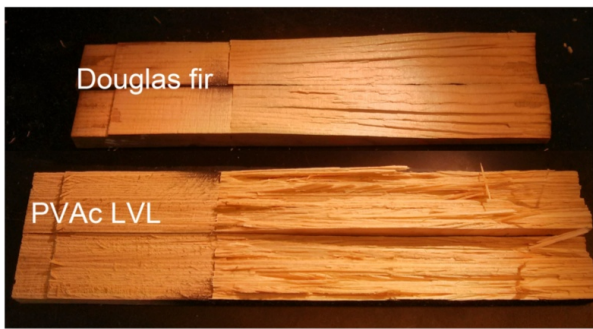
Figure 7: Fracture surfaces for DCB specimens of solid Douglas-fir wood (top) and PVA LVL (bottom) [19].
