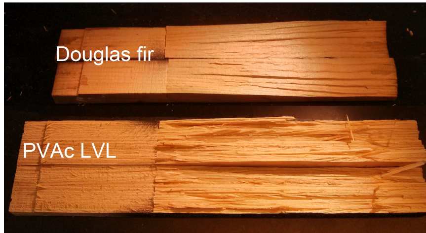
Figure 5: The fracture surface solid DF wood (top) and for DF/PVA LVL (bottom).
