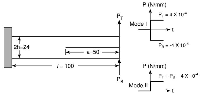
**Figure 4** : The geometry of beam specimens used to compare MPM results to static results. By varying  $P_T$  and  $P_B$ , this specimen can be pure mode I (DCB), pure mode II (ENF), or mixed mode. The loads were applied instantaneously at time zero and then held constant.
