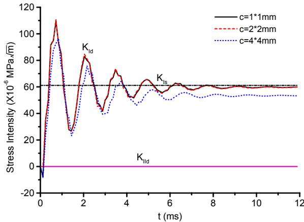
**Figure 5 :** Comparison of the stress intensity factors,  $K_I$  and  $K_{II}$ , for the DCB beam specimen calculated by MPM analysis using three different cell sizes or by analytical results (horizontal line). The dynamic MPM results had damping such that they should converge to the static solution.
