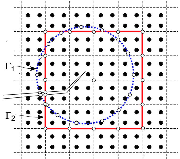
**Figure 3** : Two possible  $J$ -integral contours around a crack tip in MPM calculations. The calculations in this paper all used the rectangular path for computational efficiency. This path is centered on the node nearest to the crack tip and extends 2 cells in each direction from that node.
