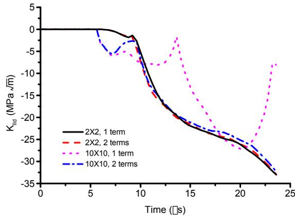
**Figure 11 :** Calculation of  $J$  integral using a line integral (one term or Eq. 7) or using a line and area integrals (two terms or Eq. 8). The calculations were for a small contour ( $2 \times 2$  cells) or for a large contour ( $10 \times 10$  cells). The results are for the mode II stress intensity factor ( $K_{II}$ ) in a DENP specimen
