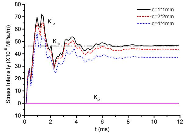
**Figure 6 :** Comparison of the stress intensity factors,  $K_I$  and  $K_{II}$ , for the ENF beam specimen calculated by MPM analysis using three different cell sizes or by analytical results (horizontal line). The dynamic MPM results had damping such that they should converge to the static solution.
