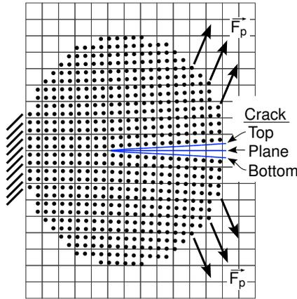
**Figure 1** : Discretization of a solid object with a crack into material points or particles. The grid is the background mesh for MPM calculations. The CRAMP algorithm tracks the crack as mass-less particles connected by line segments; it also tracks the top and bottom crack surfaces to provide information about crack opening displacement.
