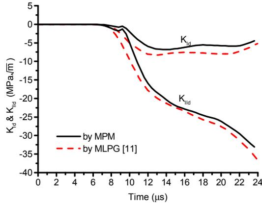
**Figure 10** : Comparison of the mode I and mode II stress intensity factors ( $K_I$  and  $K_{II}$ ) for the DENP specimen calculated by MPM or by Meshless Local Petrov Galerkin (MLPG in Batra and Ching (2002)) method.
