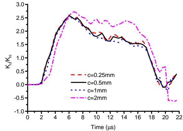
**Figure 12 :** Calculation of the mode I stress intensity factor ( $K_I$ ) in an SENT specimen as a function of the background mesh density. All calculations used a rectangular path that extend two cells from the crack tip in each direction. The background cells sizes, however, were varied using  $c = 0.25$  mm,  $c = 0.5$  mm,  $c = 1.0$  mm, or  $c = 2.0$  mm.
